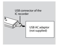
You can charge the rechargeable battery by connecting the IC recorder to an AC outlet using a USB AC adaptor AC-U50A/ AC-U50AD (not supplied).
